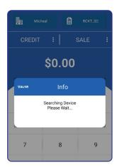
7. Upon detecting the RCKT device, a pop-up window will appear at the bottom of your screen displaying the ID of the RCKT, along with a Connect button. Click on the Connect button, and the Bluetooth icon located on the top right corner of your screen will turn green.
